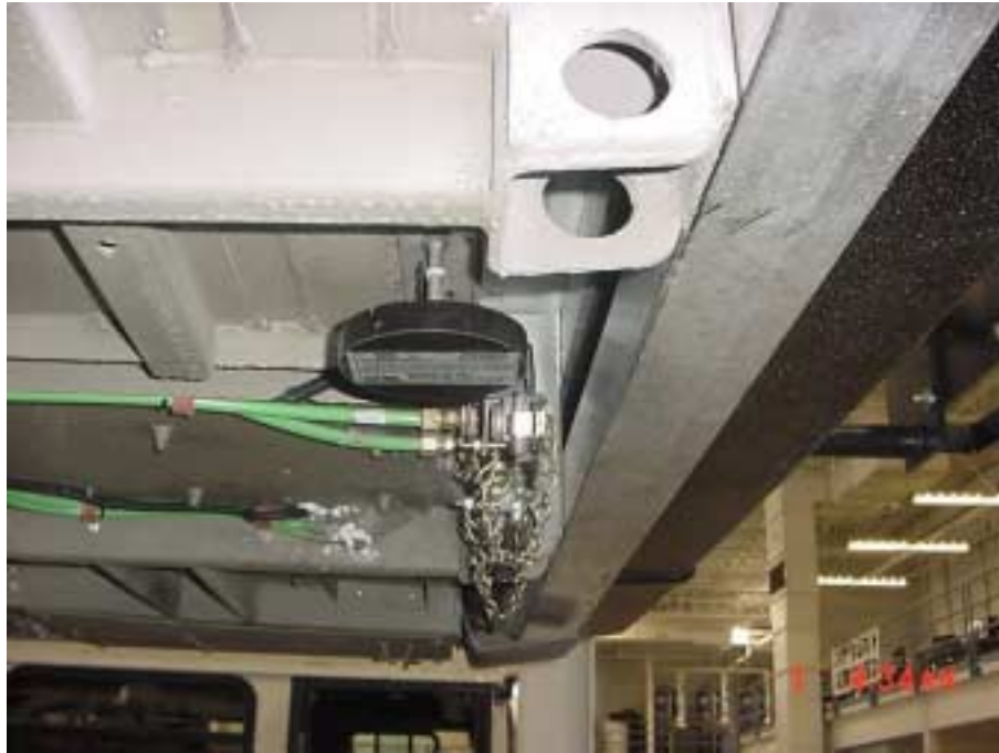
Figure 4 - Transponder Mounted on Underside of Bus
